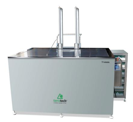
Capacity: 4000 litres Internal dimensions: 2400 x 1500 x 1325 mm. Platform dimensions: 2330 x 1350 mm. External dimensions: 2600 x 1920 x 1560 mm. Weight: 2800 kg
